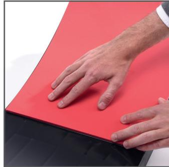
Now remove the supporting film from the EVA mat and glue them to the center of the wheel. There are about 3-4 mm of space on each side of the EVA mat. If necessary trim the last part of the EVA mat before pasting it.
