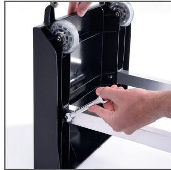
Connect the two aluminum quad tubes into the corresponding openings of the two stand modules. Fix the self-tapping screws (4.2 x 16 mm) with a 7 mm jaw wrench and a washer on the outside.
