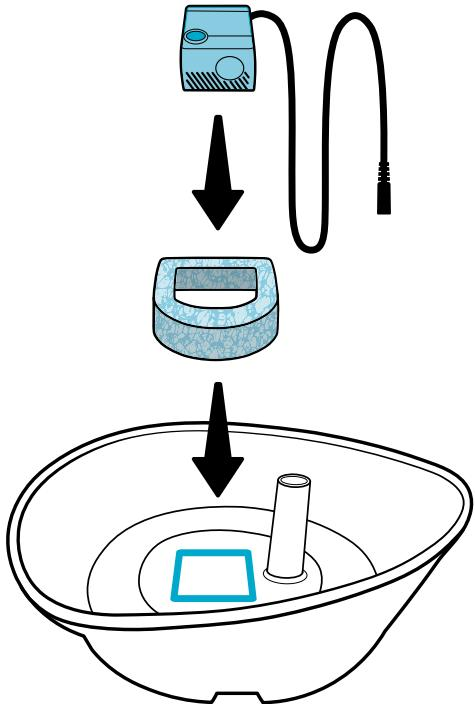
**EN** **Install the foam filter and the pump:** Insert the pump into the foam filter and set both down into the square inside the bowl. Press down to attach the suction cups.
