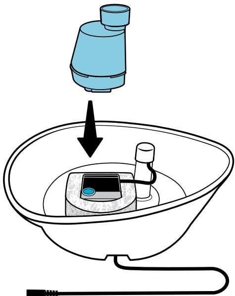
**EN** Insert the filter housing into the opening on top of the pump.
